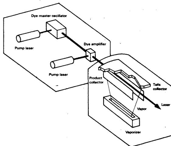
In contrast to the gaseous diffusion and the gas centrifuge methods of isotope separation, which are based on the tiny mass differences between U-238 and U-235, the Atomic Vapor Laser Isotope Separation exploits an entirely different property of the uranium isotopes: electron energies. U-238 and U-235 have different electron energies, so they absorb different wavelengths of light. AVLIS achieves the enrichment by selectively tuning in to the U-235 wavelength.
