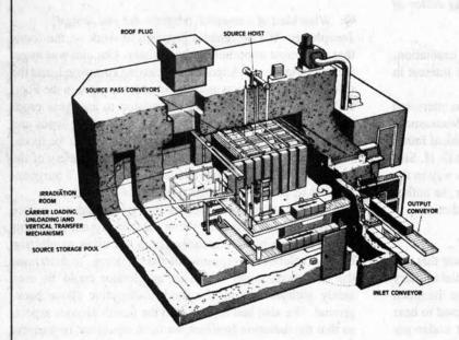
Food irradiation uses the ionizing energy from a decaying radionuclide such as cobalt-60 or cesium-137 or from srays or electron beams as a source of radiation. The very short wavelength gamma rays penetrate inside solid particles and kill microorganisms by breaking down the cell walls, or destroying their metabolic pathways.
