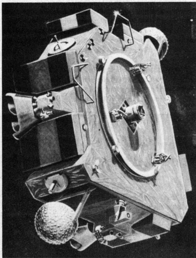
*The Orbital Maneuvering Vehicle is a reusable, free-flying space vehicle designed to enhance the Shuttle orbiter's payload delivery and retrieval capabilities. It can inspect satellites and retrieve them to a space station or the Shuttle orbiter, and can perform a variety of on-orbit tasks.*
