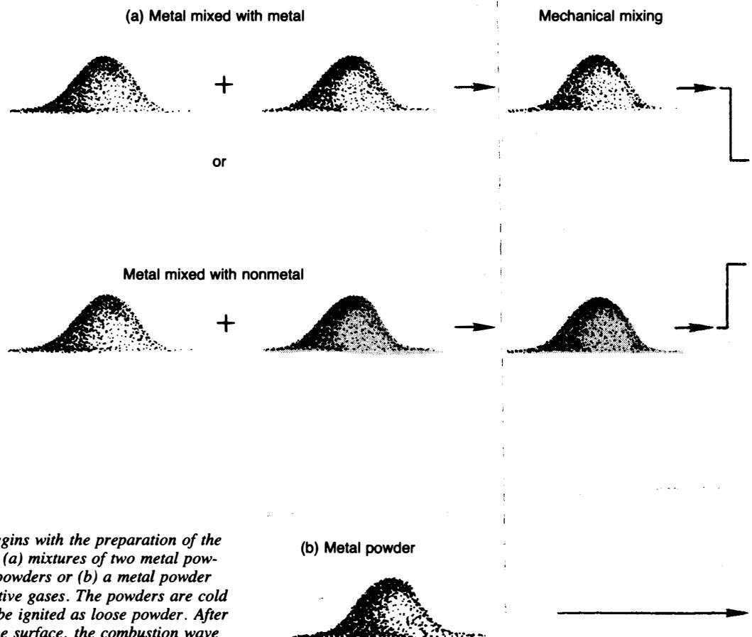
*The relatively simple process begins with the preparation of the reactants. The reactants can be (a) mixtures of two metal powders or of metal and nonmetal powders or (b) a metal powder that can be combined with reactive gases. The powders are cold pressed into a cylinder or may be ignited as loose powder. After a heated tungsten coil ignites the surface, the combustion wave moves rapidly through the material as the product is synthesized.*
