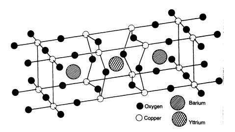
ner. Sometimes oxygens are found at other, unexpected positions in the lattice. Distortions also occur, such as in the case in which the yttrium "cube" is crushed relative to the barium cubes. This appears to occur because yttrium is smaller than barium. And that may explain why the oxygens are missing from the yttrium horizontal plane. That is, there is no room for them.
