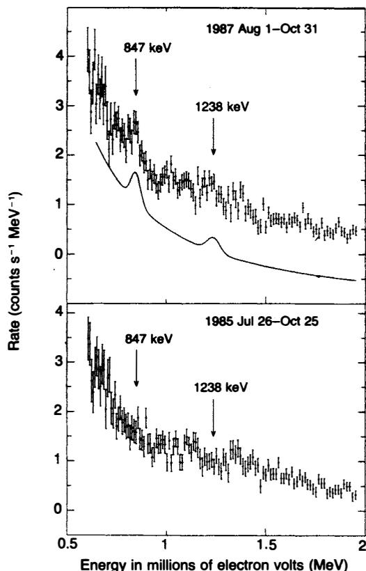
Above, a segment of the gamma-ray spectrum, recorded by the GRS from the direction of the supernova. It was accumulated over the period Aug. 1 to Oct. 31, 1987. Background flux has been subtracted, but residual atmospheric gamma-ray continuum emission remains. The solid curve is based on calculations of what we would expect to see. Below, an equivalent spectrum accumulated in 1985, for comparison.
