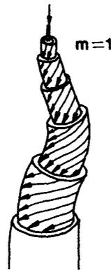
Finite conductivity model where  $B_z$  and  $B_\theta$  are mixed throughout the column
