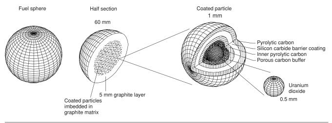
("fuel rods"), the HTR fuel elements are built from tiny, sand-corn-sized uranium "particles" which are encapsulated in concentric layers of temperature-resistant materials, including especially silicium carbide. A major advantage of these coated particles, is that nearly all the radioactive fission products, created by the fission of the uranium in the particle, remain trapped inside the particle, even at very high temperatures.
