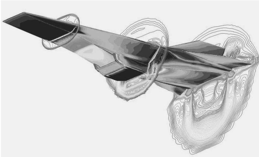
*Beyond a speed of Mach 8, where the ability to test in wind tunnels is lost, scientists use computational fluid dynamics to analyze air flow and shock fronts around hypersonic aircraft. This is such a diagram of the Hyper-X.*
