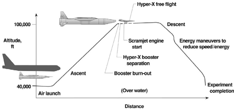
*During a flight test of the Hyper-X, or X-43, a B-52 flies to 40,000 feet, where it releases the X-43, which is attached to a Pegasus rocket. The rocket ascends to 100,000 feet, and the X-43 flies using its scramjet engine after release from the Pegasus.*
