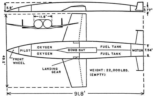
A diagram of Eugen Sanger's anti-podal bomber, which would be capable of travelling halfway around the world and landing at an airport.
