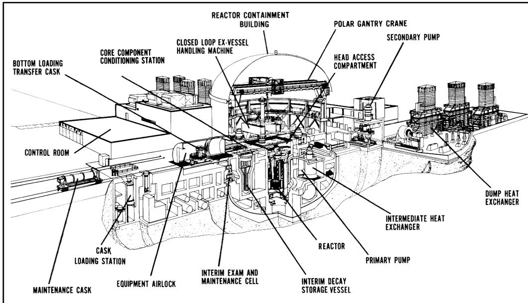
*The FFTF is a liquid-sodium-cooled reactor with a fuel of mixed uranium oxide and plutonium oxide. Fast flux refers to the speed of neutrons produced in the reactor core during the fission process. The reactor vessel is located in the dome-shaped containment building.*
