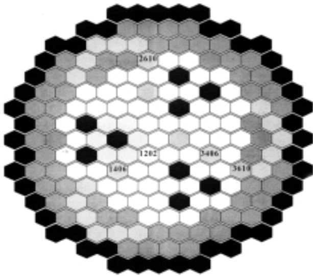
*This schematic of the FFTF core with multiple missions shows the hexagonally shaped ducts, in which multiple experiments can be conducted. Some ducts contain the fuel rods and control rods. Others are for isotope production, fuel tests, and so on.*
