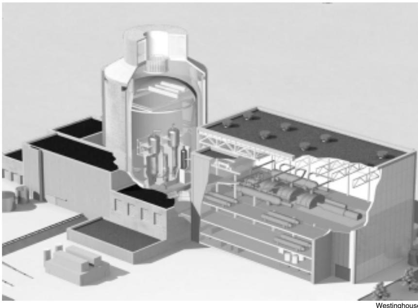
*A cutaway view of the next generation Westinghouse AP 1000 reactor, which has been designed with approximately 600 modules. This approach will allow converting sections of the auto industry into building modular components for new nuclear plants, as well as other much-needed infrastructure.*
