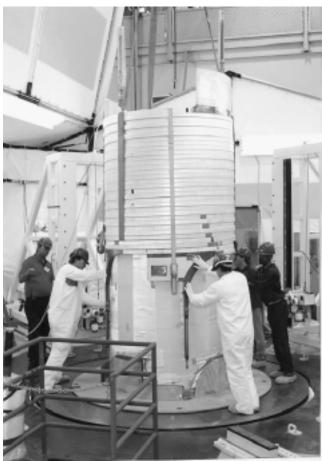
One of the technological challenges of building the ITER tokamak is a series of superconducting magnetic coils, that must be kept at temperatures near absolute zero. To develop new manufaturing techniques to accomplish this, test components have been created, such as this section of a central solenoid, which was made in the United States by Lockheed Martin, and then shipped to Japan for testing.
