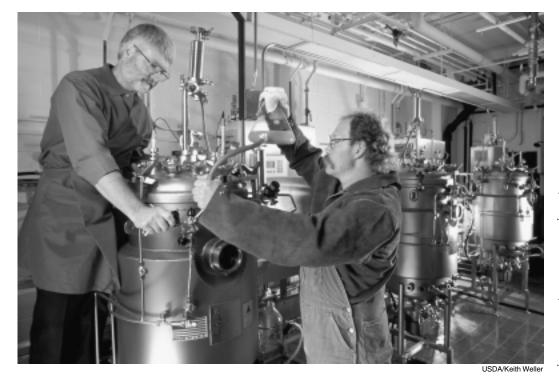
In a scene straight out of an H.G. Wells film, a microbiologist and technician add starter microorganisms to pilotplant-size bioreactors in which ethanol is brewed from sugar mixtures derived from corn fiber. "The vision is of ethanol stills dotting the rural land area, drawing on the labor of hardworking peasants in a production radius of 25-30 miles for corn stover, and up to 60 miles for plants using switchgrass as a feedstock.'
