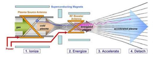
Ad Astra's diagram of the VASIMR Rocket. The Plasma Source cell involves the main injection of a neutral gas like hydrogen to be turned into plasma and the ionization subsystem. The RF Booster cell uses electromagnetic waves to energize the plasma to the desired temperature. The Magnetic Nozzle then converts the plasma energy into directed motion and ultimately useful thrust.
