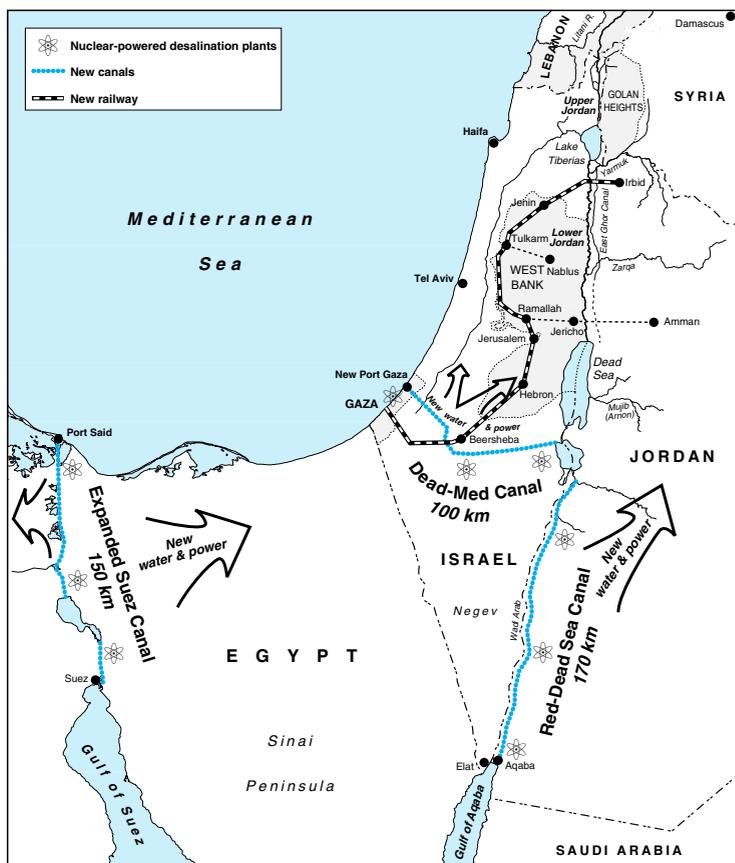
But the idea then is, from the Red Sea, to build a canal, which goes downwards to the Dead Sea, and you can use the difference in elevation for hydropower. The idea was to desalinate water with that power, which Jordan needs a lot. That project is dead. It doesn't exist anymore because of all these political destabilizations. But the engineers are ready to build it.
