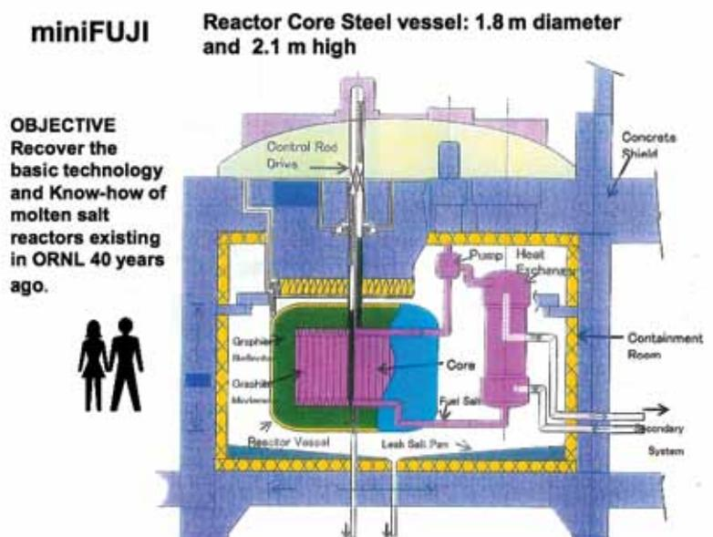
two places at the bottom where, if you drain the fuel, it goes down there and becomes completely harmless, because the fuel only produces fission when it is inside with graphite. If the fuel flows out, it is harmless. When it cools, it becomes like a stone. On the right side, are the parts of the reactor that are to transport energy and heat, and thus to produce electricity.
