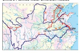
water from a tributary of the Yangtze River to Beijing; and, the Western route is taking water from near the Tibetan plateau, by diverting water from the Yangtze River to the Yellow River.
