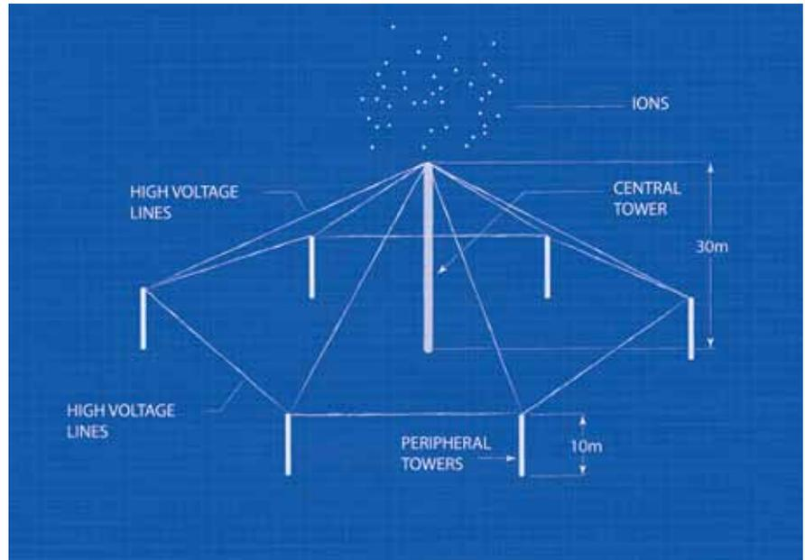
*This is a simple schematic of the ELAT system, one of the ionization technologies used to affect the electrical conditions of the atmosphere which contribute to rainfall. Similar systems are currently, or have previously been used across the globe, and have shown promising results in our ability to modulate rainfall in a targeted way.*
