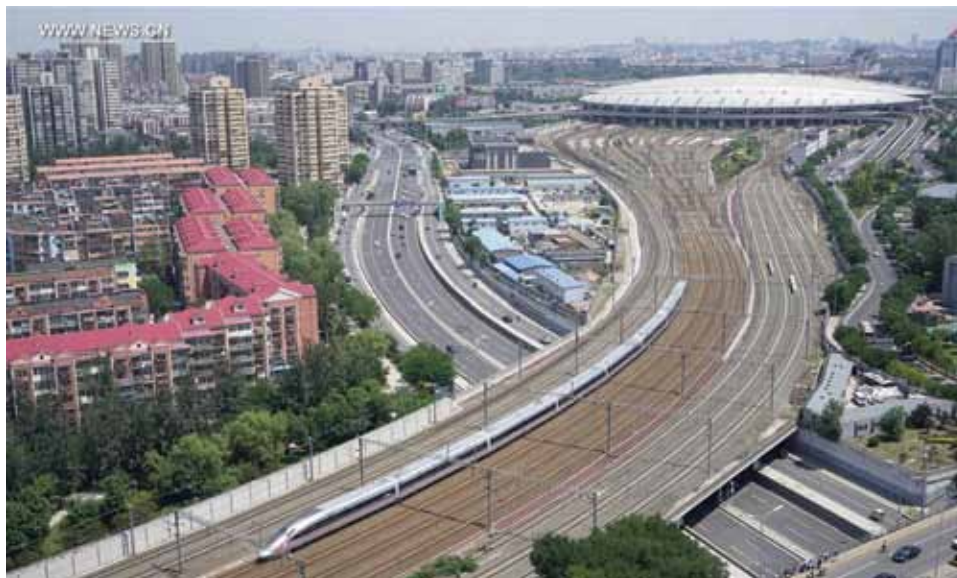
China’s new bullet train “Fuxing,” pulling out from Beijing South Railway Station, June 26, 2017. The new-generation train has a top speed of 400 kilometers an hour, and a consistent speed of 350 km an hour.
