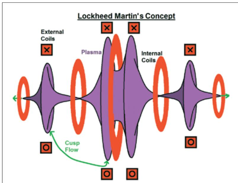
*Conceptual schematic of Lockheed Martin’s truck-sized high-beta compact fusion reactor.*
