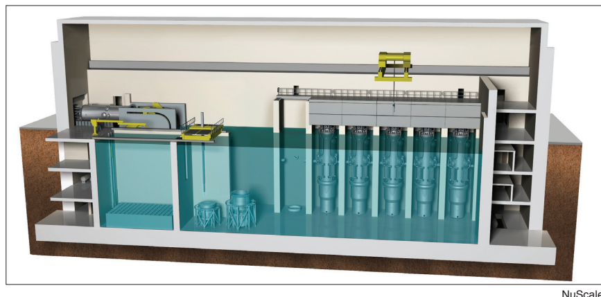
Artist’s rendering of a cross-section of a NuScale SMR power plant, showing five reactor modules installed in a below-grade pool of cooling water: NuScale’s 60 MW reactor modules are designed to be installed individually or in arrays of up to 12 units in a single plant.
