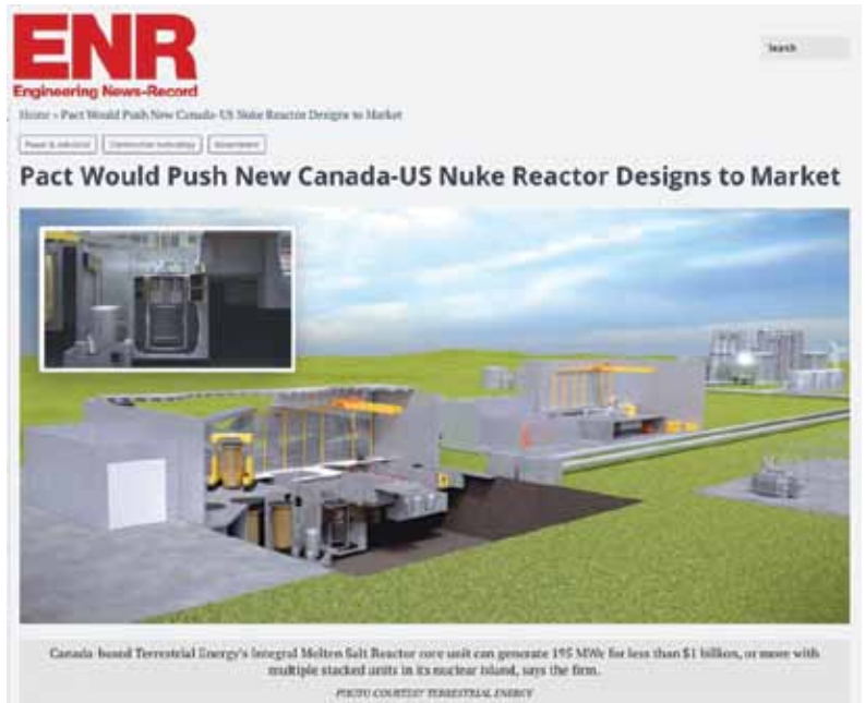
Artist's depiction of Canada-based Terrestrial Energy's Integral Molten Salt Reactor; employing Generation IV molten-salt technology, with a power output of 195 MW. Multiple reactor modules can be stacked in its nuclear island.
