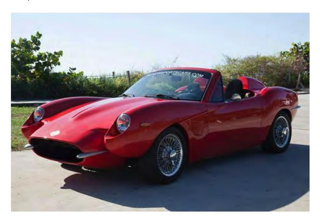
An entrepreneur in Florida built a sports car out of hemp. Called the Renew Sports Cars, this hemp car comes out to be 4.7X greener than even an electric car. Similar to Henry Ford's car, this car's exterior is all made from hemp plastic and it runs on hemp biofuel.
