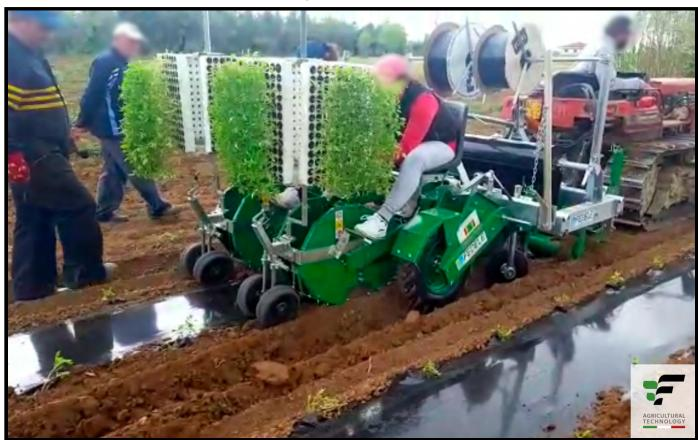
Flagship of Fedele, the combined Transplanter - Mulching machine, specifically designed for halving working time and relative labour costs through the simultaneous execution (in one step) of 4 basic operations:
