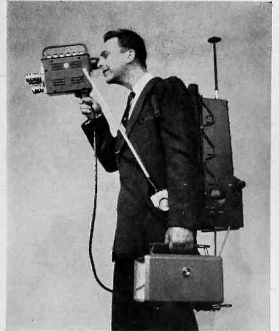
*Well-known news commentator Chet Huntley carries a portable TV camera and back-pack transmitter, two-way "transceiver" for radio communication (in pocket) and a light portable TV set.*
