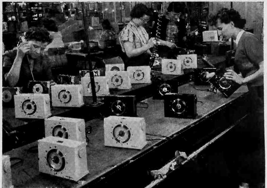
*Clock-radios being carefully tested and prepared for shipment.*
