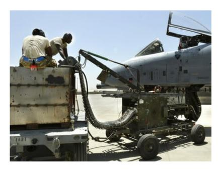
A-10 being loaded with 30mm PGU-13/B high explosive incendiary (HEI) ammunition in Afghanistan. It can fire either HEI alone, or its standard combat load, which is a mixture of HEI and DU armour piercing incendiary (API) ammunition. It cannot select between ammunition types once airborne, one of the reasons why DU has historically been used against a far wider range of targets than just tanks.
