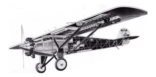
See, no weight in the rear. Main gas tanks in these small monoplanes were normally in the rear, and that wasn't just because that was where the free space existed. It was to balance the plane forward and back. To fly, this plane has to be balanced, with a center of gravity somewhere beneath the line of the wings. A rear gas tank balances the heavy engine in the front. That is especially true at take-off, when the nose has to be in the air for angle of attack.
